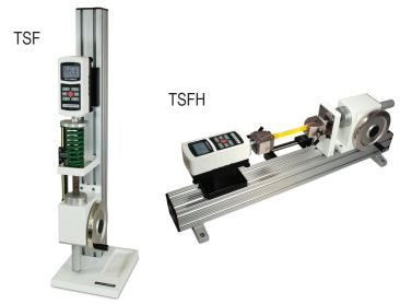
The TSF is shown testing a compression spring, with a Series 5 digital force gauge and digital travel display
