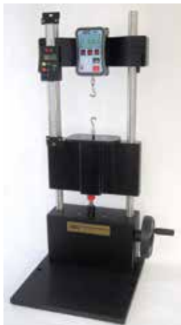
Force One™ FDIX mounted on Wagner FTK 200 Spring Tester
